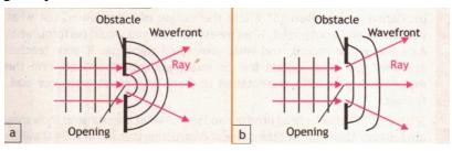
After passing through the opening, waves spread out in every direction and turn into circular waves. This effect is greatest when the size of the opening is less than or equal to the size of the wavelength of generated waves. It must be noted that wavelength (or speed) of the wave is not affected by diffraction.
