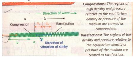
compressed together (called compression) is seen moving towards the right. The region where the part of slinky are stretched apart (called rarefaction) is also seen moving towards the right.
