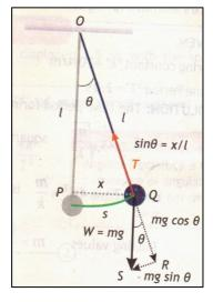
The component "mg  $\cos\theta$ " is balanced by the tension "T" in the string. The restoring forces only provided by component "mg  $\sin\theta$ ". Therefore
